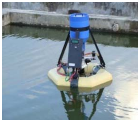
FIGURE 1 – A WATER QUALITY MEASUREMENT SYSTEM PROPOSED BY [4].
