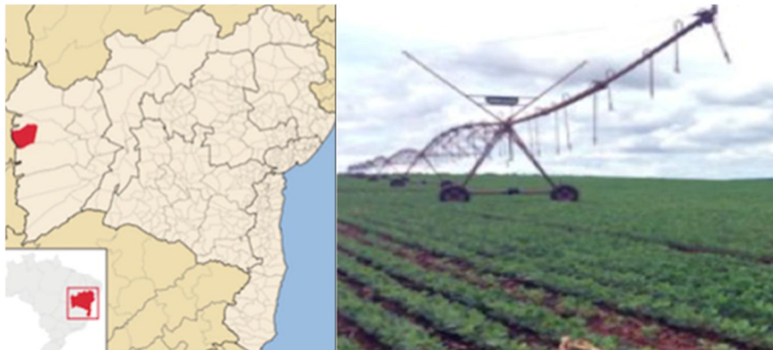
FIGURE 8 - CENTER-PIVOT IRRIGATION PILOT: LOCATION OF THE PILOT SITE (LEFT) AND CENTER PIVOT IRRIGATION FOR SOYBEAN CROP (RIGHT)
