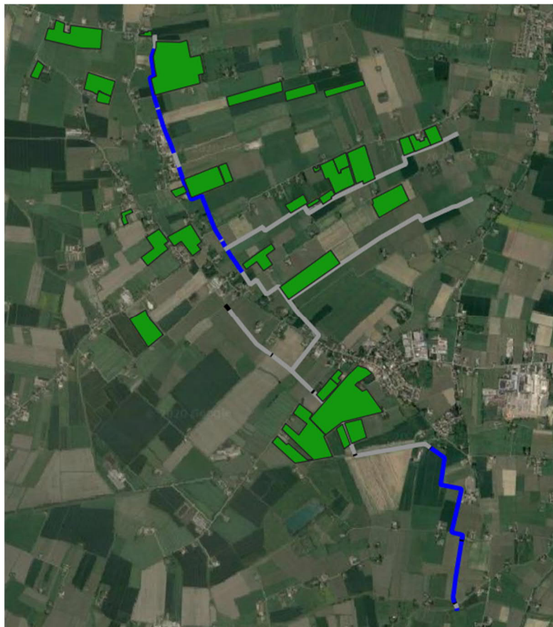
FIGURE 5.1: PILOT IRRIGATION DISTRICT OF CBEC, IN BLUE OPEN CANAL, IN GREY PIPES, IN GREEN IRRIGATED FARMS IN 2019
